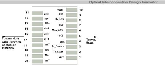
Figure2.Electrical Pin-out Details
